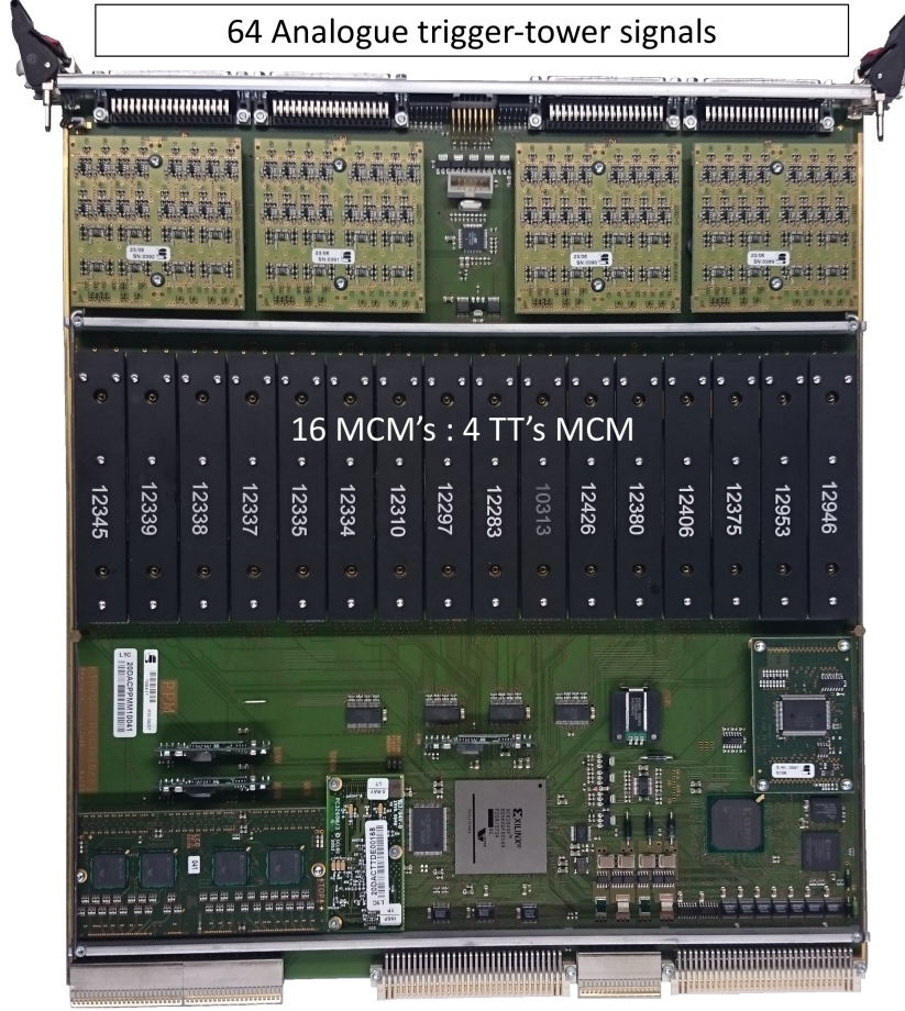
Figure 4.3: Photograph of a PreProcessor Module [3]. These modules host 16 MCMs where the main processing of the signal takes place.
