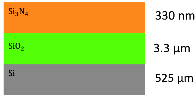
Figure 4: Layer stack of a PIC, comprising of silicon nitride ( \text{Si}_3\text{N}_4 ), silicon dioxide ( \text{SiO}_2 ), and silicon ( \text{Si} ).
