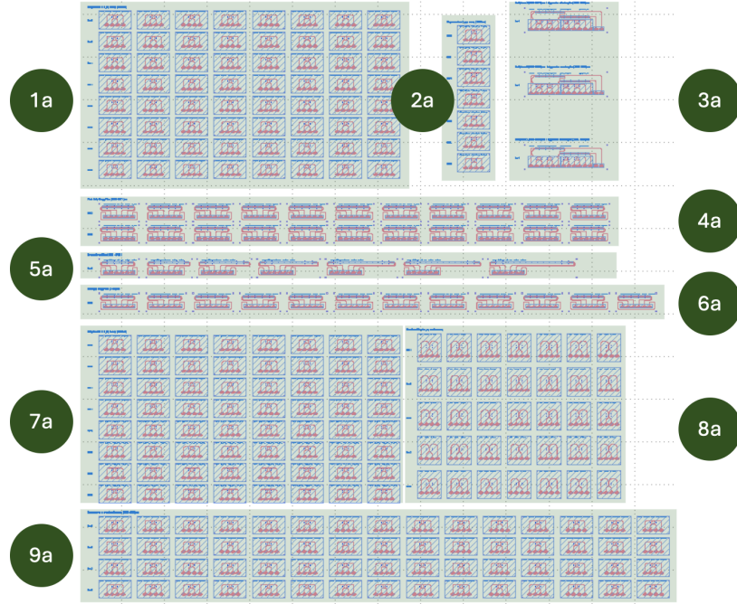
Figure 21: Illustration of the first chip, on which parameter sweeps were conducted for ring resonators, Bragg filters, and directional couplers across various sections, along with the construction of test multiplexer structures. The different sections are labeled, and these labels are subsequently referenced.
