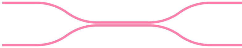
Figure 4: Illustration of a directional coupler with a length of 30\ \mu\text{m} , a gap of 0.5\ \mu\text{m} , a waveguide width of 1.2\ \mu\text{m} and a bend radius of 30\ \mu\text{m} .
