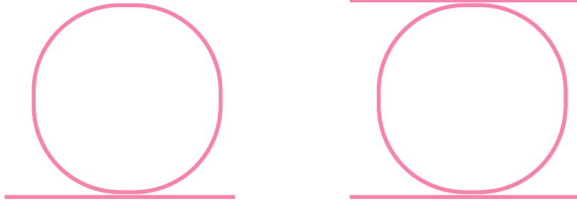
Figure 6: Illustration of two ring resonators. On the left, an all-pass ring resonator, and on the right, an add-drop ring resonator. Both are racetrack ring resonators with a horizontal and a vertical straight region. The dimensions here are: waveguide width = 1.2 \mu\text{m} , resonator radius = 30 \mu\text{m} , gap = 0.5 \mu\text{m} , and straight length = 5 \mu\text{m} (horizontal and vertical).
