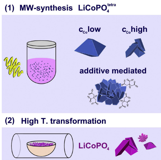
Fig. 1. Schematic of the two step synthesis: microwave-assisted hydrothermal synthesis of \text{LiCoPO}_4^{\text{tetra}} and high temperature transformation to \text{LiCoPO}_4 .
